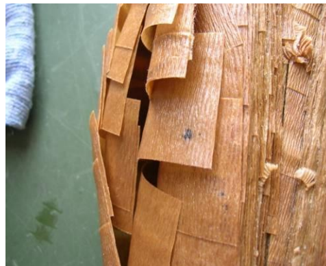
Degradated oil/paper insulation
