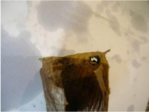
Degradated oil/paper insulation
