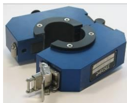
HFCT clamped around cable ground lead
